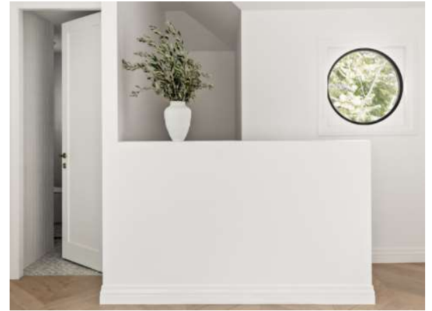
1200mm high dwarf wall to both flight and first floor.
